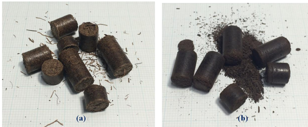
Figure 4-11. The appearance of the pellets after tumbling; (a) HTT-180 hydrochar pellet and (b) HTT-220 hydrochar pellet
