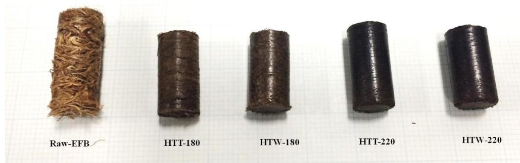
Figure 4-5. The appearance of the pellets made from raw-EFB, hydrochars and washed hydrochars
