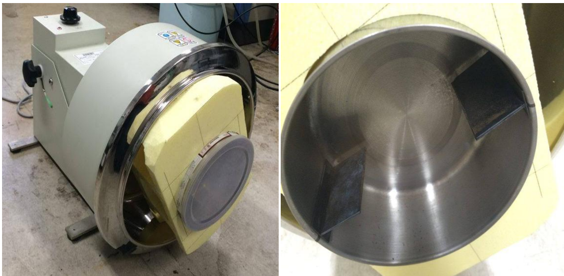
Figure 4-2. The tumbler can set up in the laboratory
